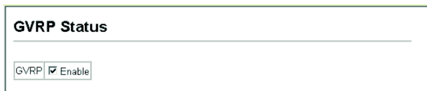
Figure 3-61 Globally Enabling GVRP
